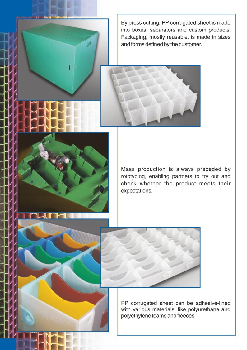
PP corrugated boxes are designed to be durable and to fold flat. The latter is an important feature for boxes that are often transported or stored empty during their long lifetime, because it minimizes the space they occupy. Non-self-closing boxes are closed by metal clips, plastic rivets or ultrasonic welding.
